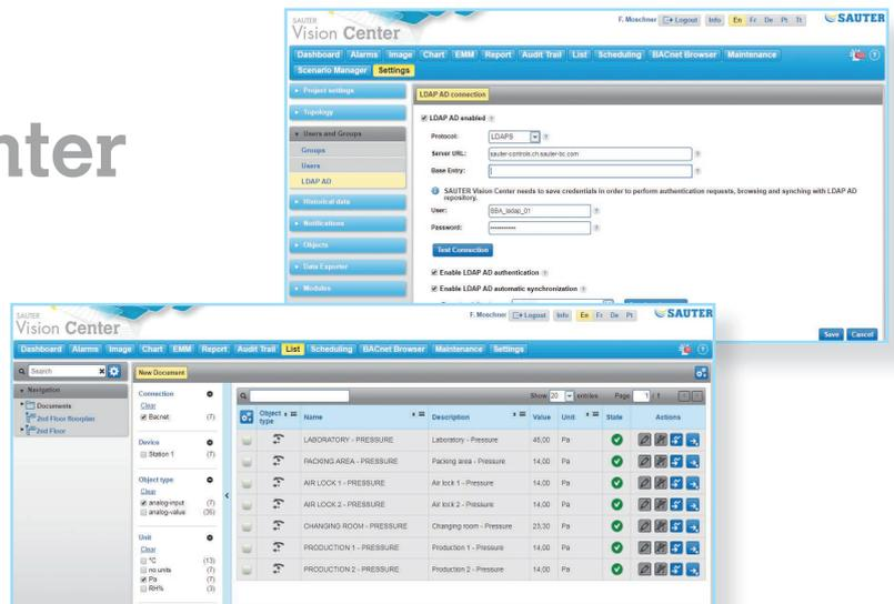
Facilitating preventive service deployments means that the solution helps detect sources of errors at an early stage. This reduces the risk of malfunction. The data recorded also generates valuable information, enabling maintenance schedules to tie in with actual operation. This keeps service deployments and the cost involved to a minimum.
