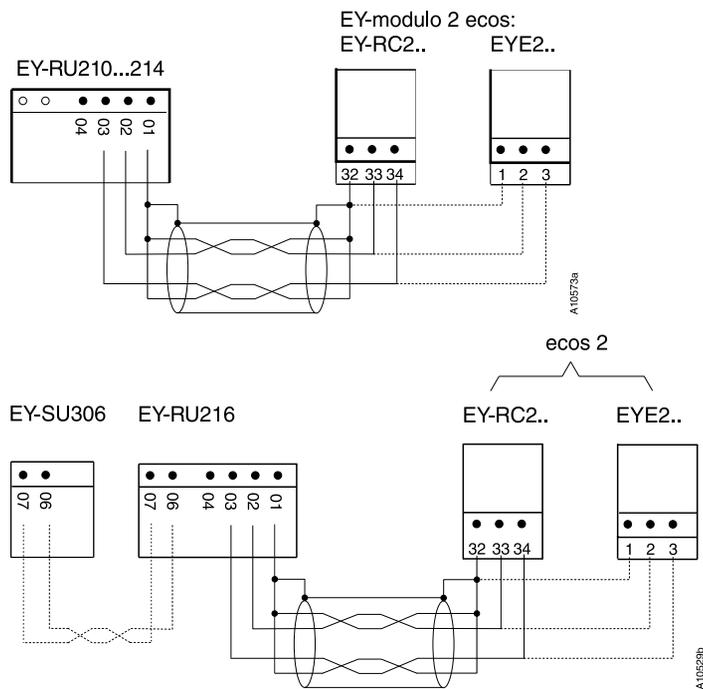
The resistance to interference of the transmission between the operating unit and the ecos is increased by using twisted connecting cables.
