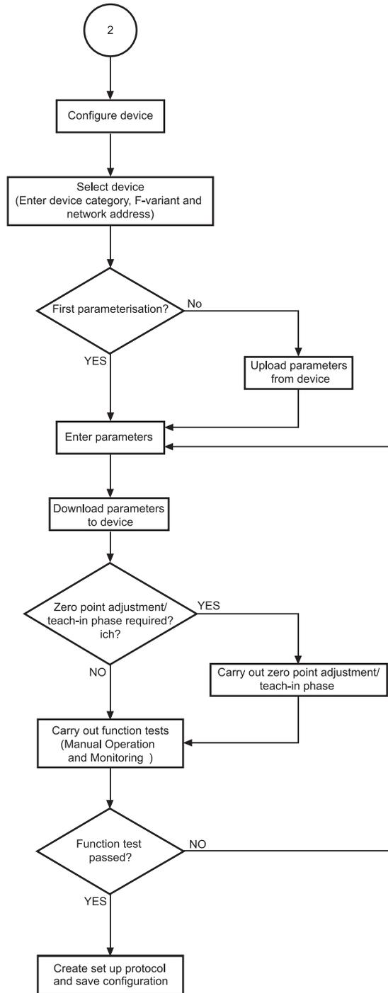
Fig. 1 Configuration flowchart
