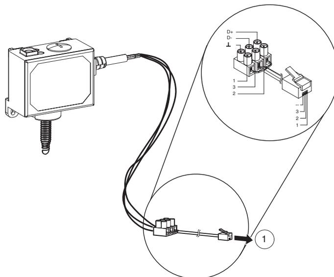
Fig. 6 Connection of SGU100 with clamp terminal
