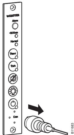
Fig. 14 Separating the connection between SGU100 and PC (connection via 3-pin plug connection on the FCCP)
