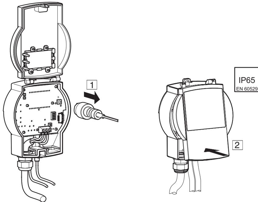
Fig. 12 Separating the connection between EGP100 and PC (connection via 3-pin plug connection)
