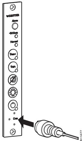
Fig. 7 Connection with an SGU100 via 3-pin plug connection on the FCCP
