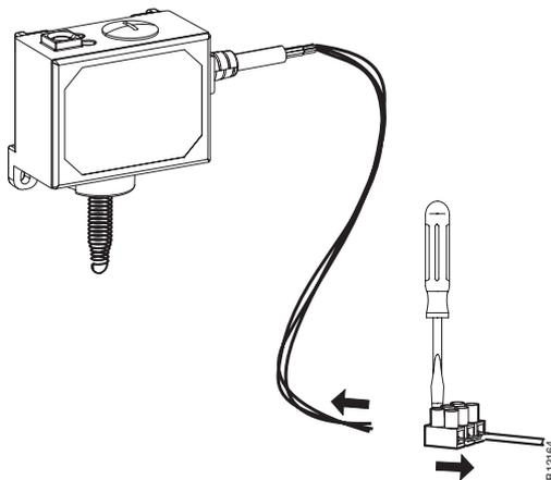
Fig. 13 Separating the connection between SGU100 and PC (connection via terminal block)
