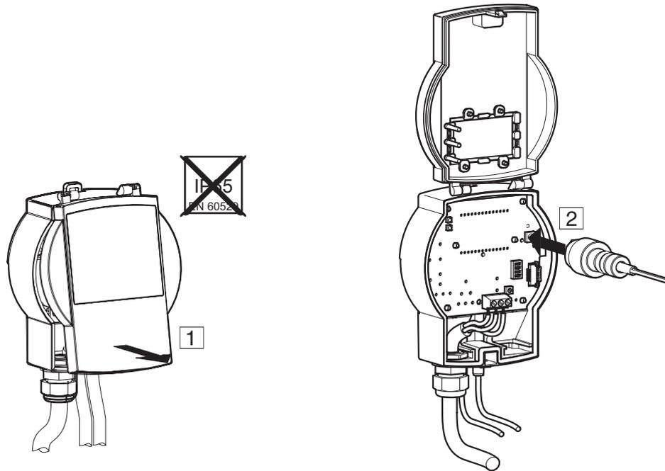
Fig. 5 Connection with an EGP100 via 3-pin plug connection
