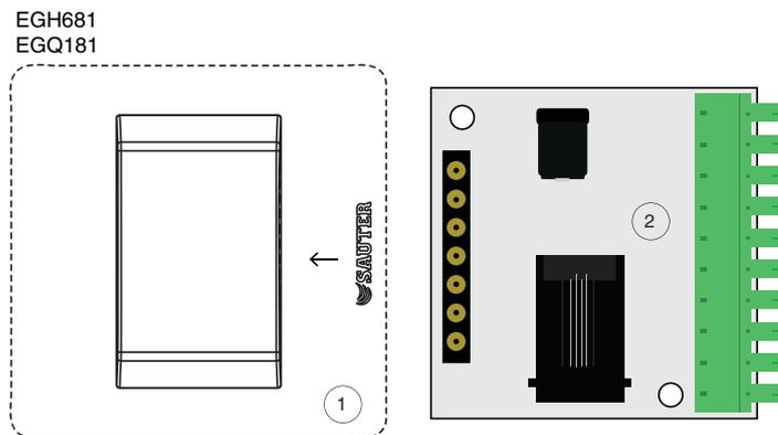
Fig. 15 Separating the connection between EGQ181SF203 and universal converter, separating the connection between EGH681SF233 and universal converter
