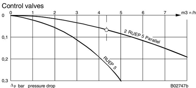
In order to estimate the total pressure drop, the air throughput rate  $\dot{V}_{max}$  is determined according to 4.2) and the relevant  $\Delta p$ -values of the corresponding load curves are added up:
