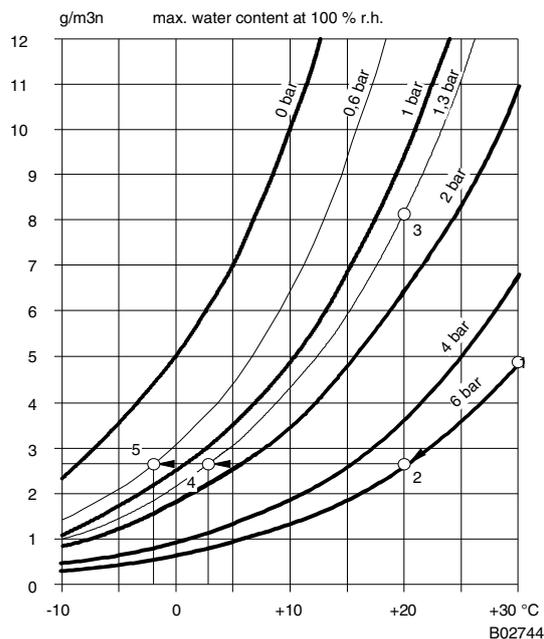
The high-pressure network is intentionally used for water separation
