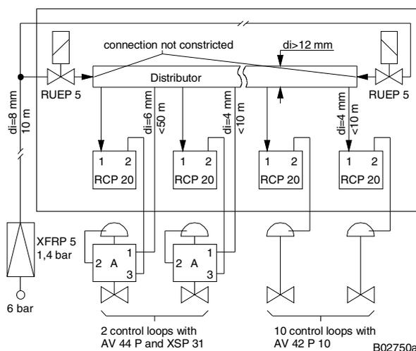
Typical air throughput  $\dot{V}_{max}$  at the distributor (see section 4.2)
