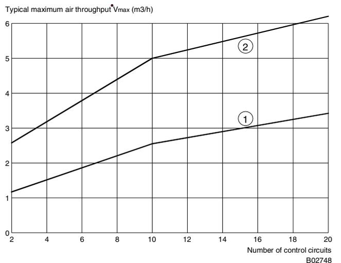
When a complete installation is switched on or when a common setpoint adjustment is carried out, larger quantities of air are required for short periods, i.e. the permissible supply pressure variation is exceeded. The resulting influence on the devices as detailed in 4.3) is usually permissible for these cases.
