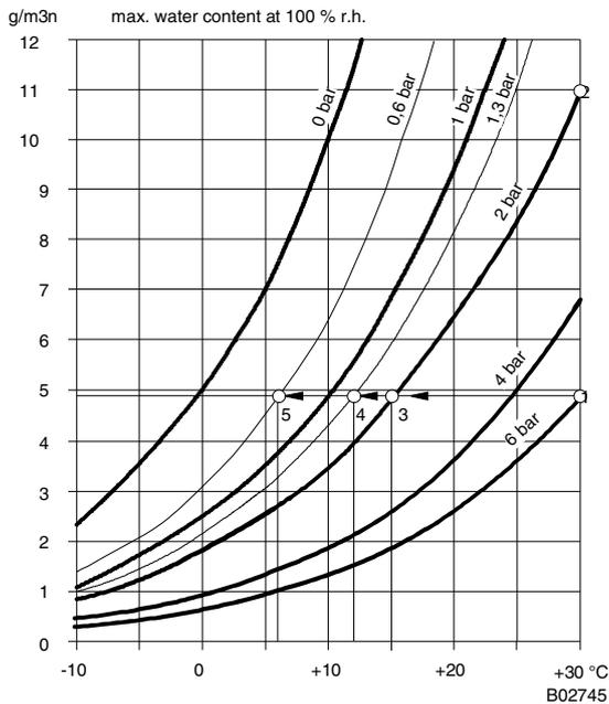
The initial pressure reduction in the compressor chamber reduces the rel. humidity in the high-pressure network. Due to the reduced „high pressure”, the line pressure drop is increased and the performance of the second reduction unit is decreased.
