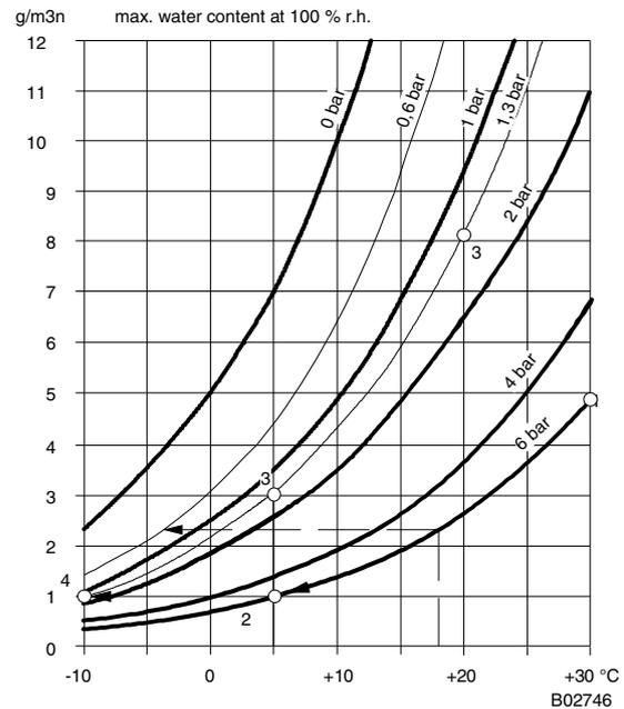
The compressed air (6 bar) is cooled and a corresponding amount of water separates. With water coolers, approx. 18 °C and, with refrigerating machines, approx. 5 °C can be attained (limited by the freezing point).
