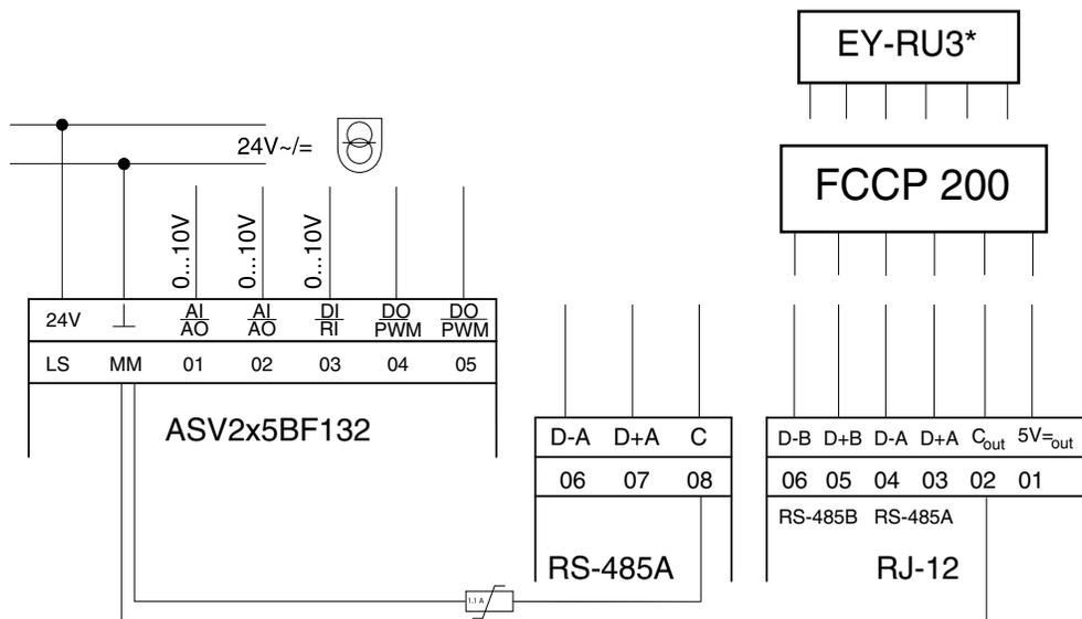
Block diagram for VAV.01.101.M (factory setting)
