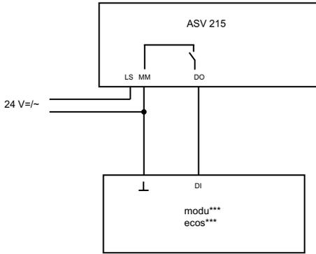
The MM terminal of the ASV 2\*\* to be connected must be connected to the ground of the ecos500 and the modu525.
