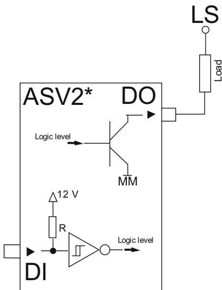
**Connection of DO ASV to DI AS, RC**
