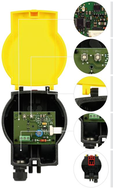
Exact measurement using a double-membrane pressure sensor: this high-calibre sensor will even detect the most minimal air flows or differential pressures. A differential capacitive method of measurement is used to evaluate the differential pressure and make it available in the form of a linear electrical signal. Another advantage of the membrane sensor is that it can be fitted in any position
