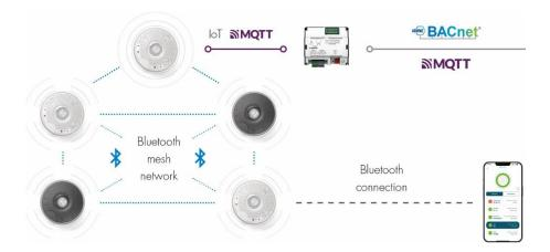
IoT for future-oriented room automation: Wireless communication between sensors and system integration via MQTT.
